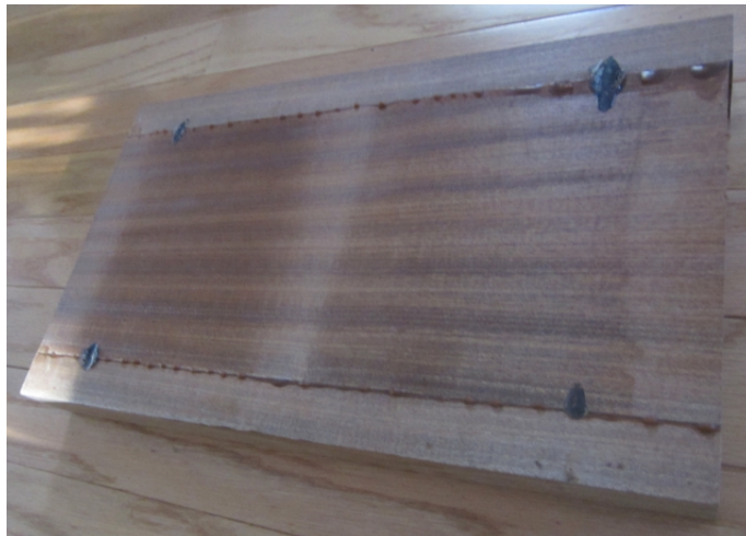
Photo Two After the Glue Dried but Before Planing
